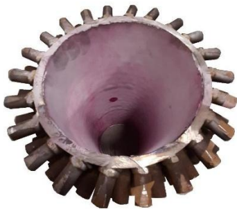
Figure 2: Pipe sample with dye penetrant inspection
