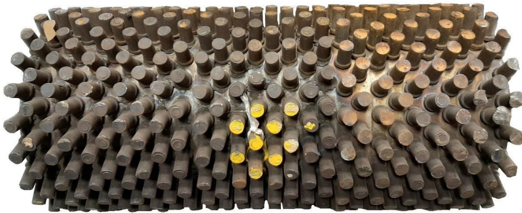
Figure 1: Studded pipe sample, as received
