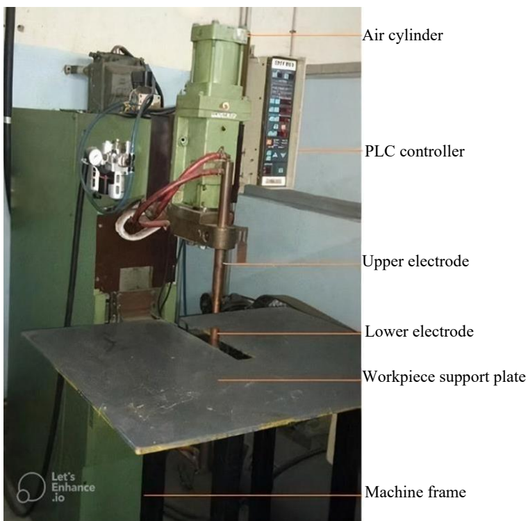
Figure 4. Electric resistance spot welding machine setup.
