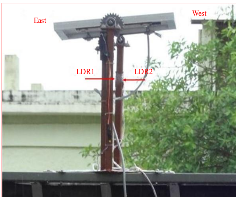
Figure 2. Light intensity variation measurement setup.
