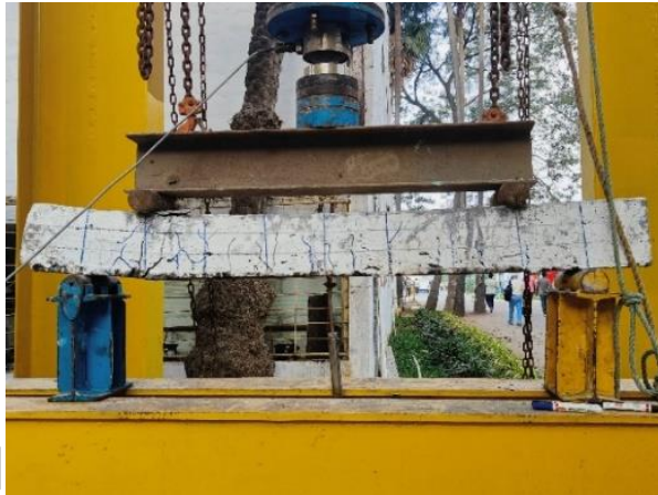
Figure 24. Experimental setup for test beams with different concrete mixes. (a) Conventional concrete(N1) (b) Optimum mix concrete(A1).
