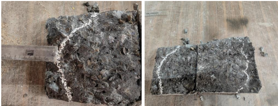
Figure 13. Measuring the depth of water penetration into concrete specimens at water permeability test.
