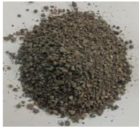
Figure 3. Fine steel slag.
