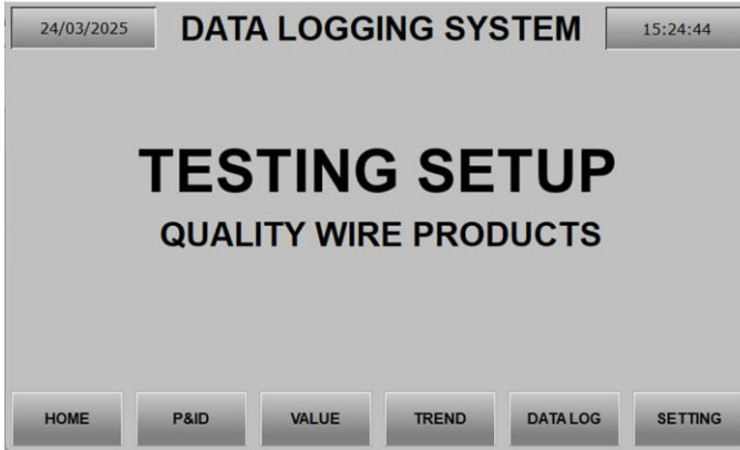
Fig. 4. HMI Screen – Home
