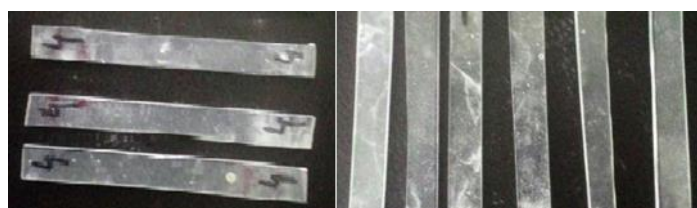
Figure 1. Photograph of the fabricated HNT/epoxy composite specimens.
