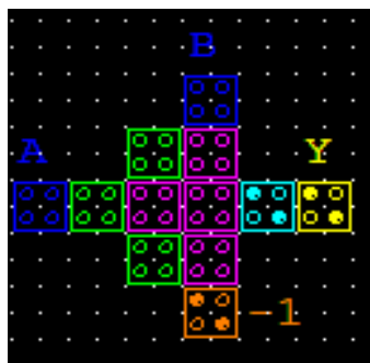
Figure 4. Implementation of 2-input Ex-OR Gate
