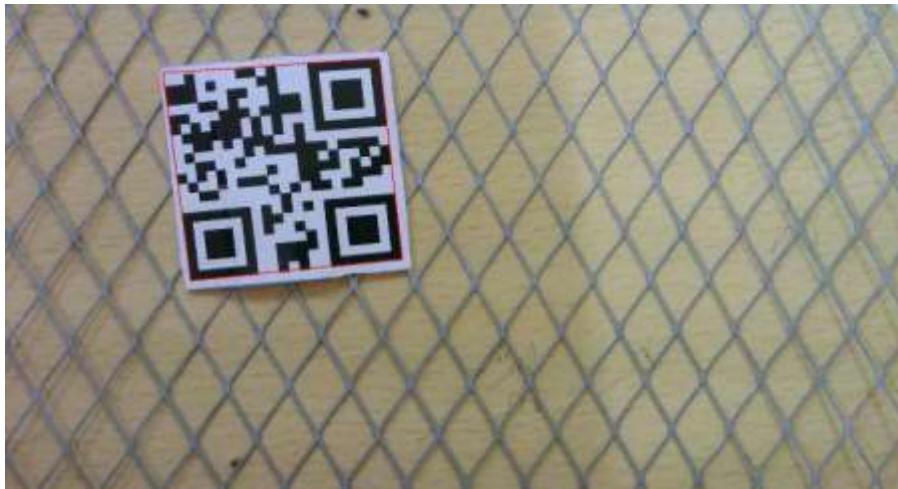
Figure 8. QR Calibration Target Co-Planar with a Woven GF/EP Specimen on a Contrasting Background. The Red Bounding Box Confirms Successful QR Detection for Session Calibration.
