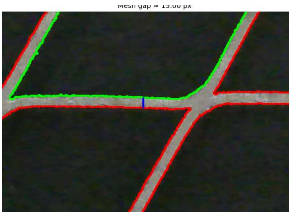
Figure 6. Inter-Tow Gap Measurement Visualisation. Green Overlay: Primary Tow Boundary; Red Overlay: Adjacent Tow Boundary; Blue Line: Measured Perpendicular Gap T .
