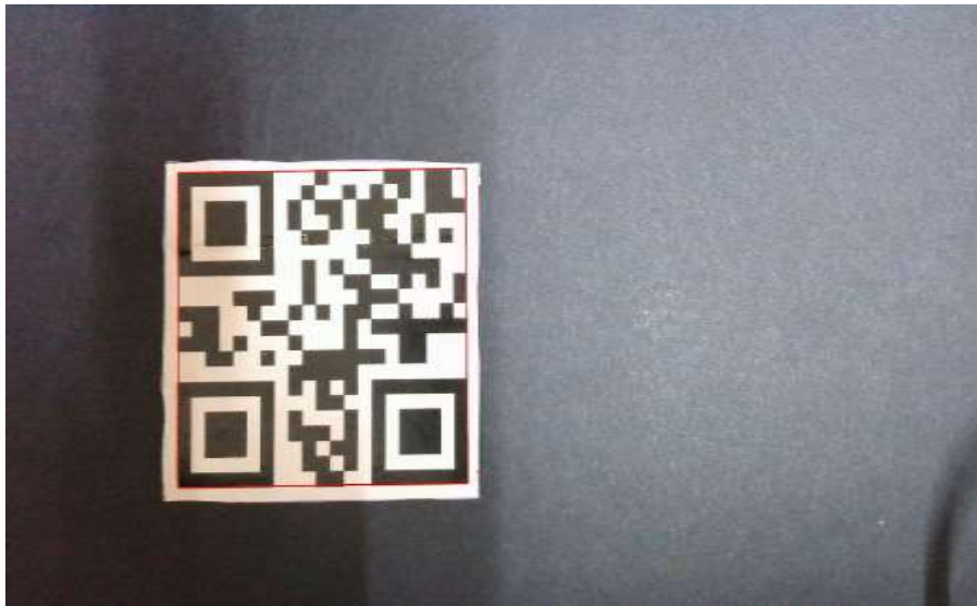
Figure 7. QR Code Reference Target Used for Pixel-to-Millimetre Calibration. Red Bounding Box Shows Detected QR Boundaries; Physical Width W_{\text{mm}} = 39 mm Provides the Calibration Reference.
