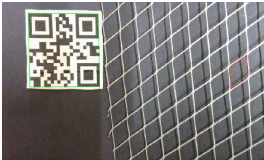
Figure 3. Imaging Setup Showing the Co-Planar QR Calibration Target (Green Bounding Box) Alongside the Woven Composite Specimen. A Detected Unit Cell Is Highlighted with a Red Polygon Overlay.
