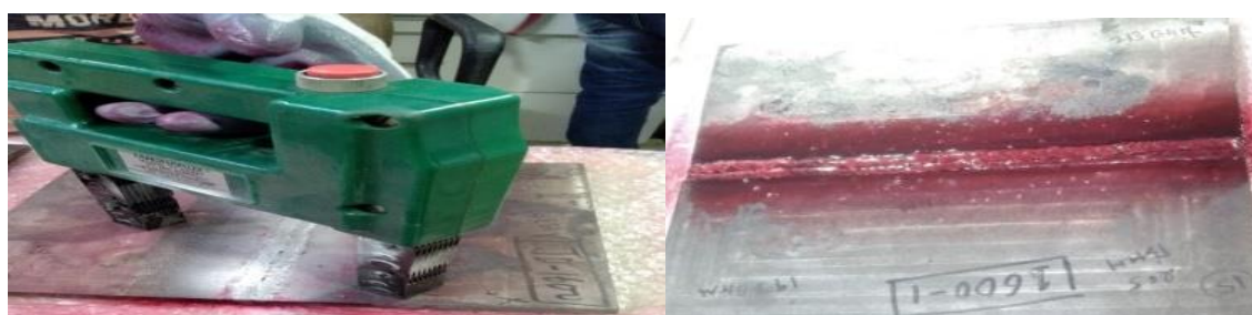
Figure 6. MPI & DPT of 9 welded plate
