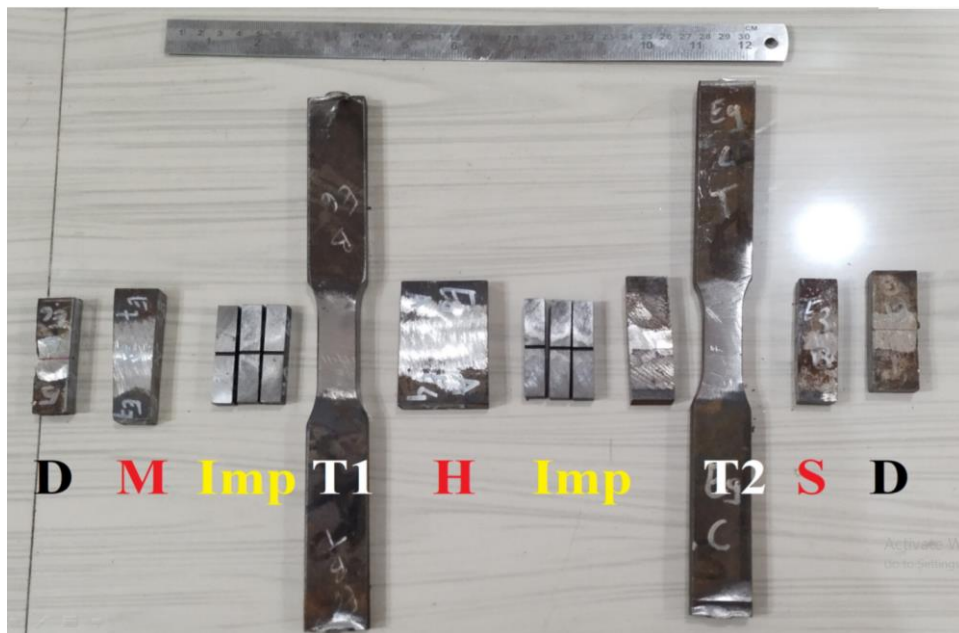
Figure 4. 300 * 300 *12 Mm welded plate cut into different testing samples
