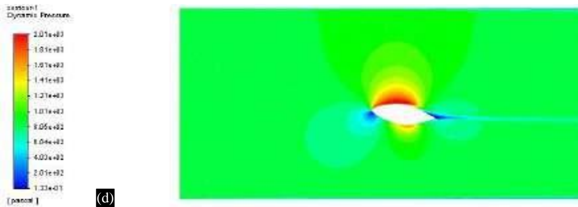
Figure 10. Pressure contour at 8° angle of attack (at 37 m/s). (a) Javaplum leaf, (b) Ixora leaf, (c) Custard apple leaf, (d) Sapota leaf
