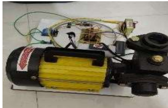
Figure 9. ESP32-Based motor monitoring system1.
