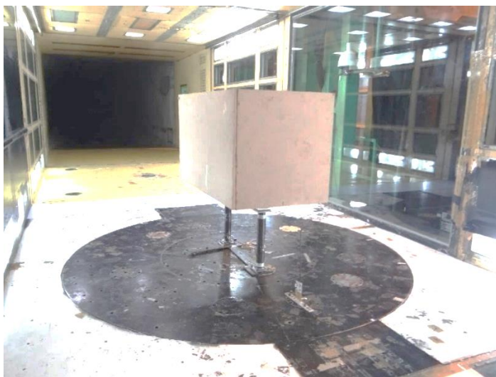
Figure 17. Scaled bus wind tunnel model.
