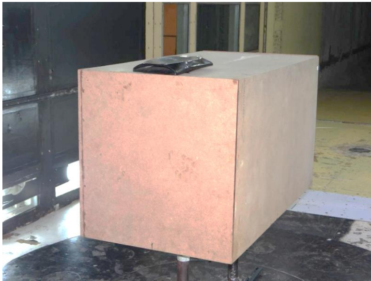
Figure 18. Scaled bus & device wind tunnel model.
