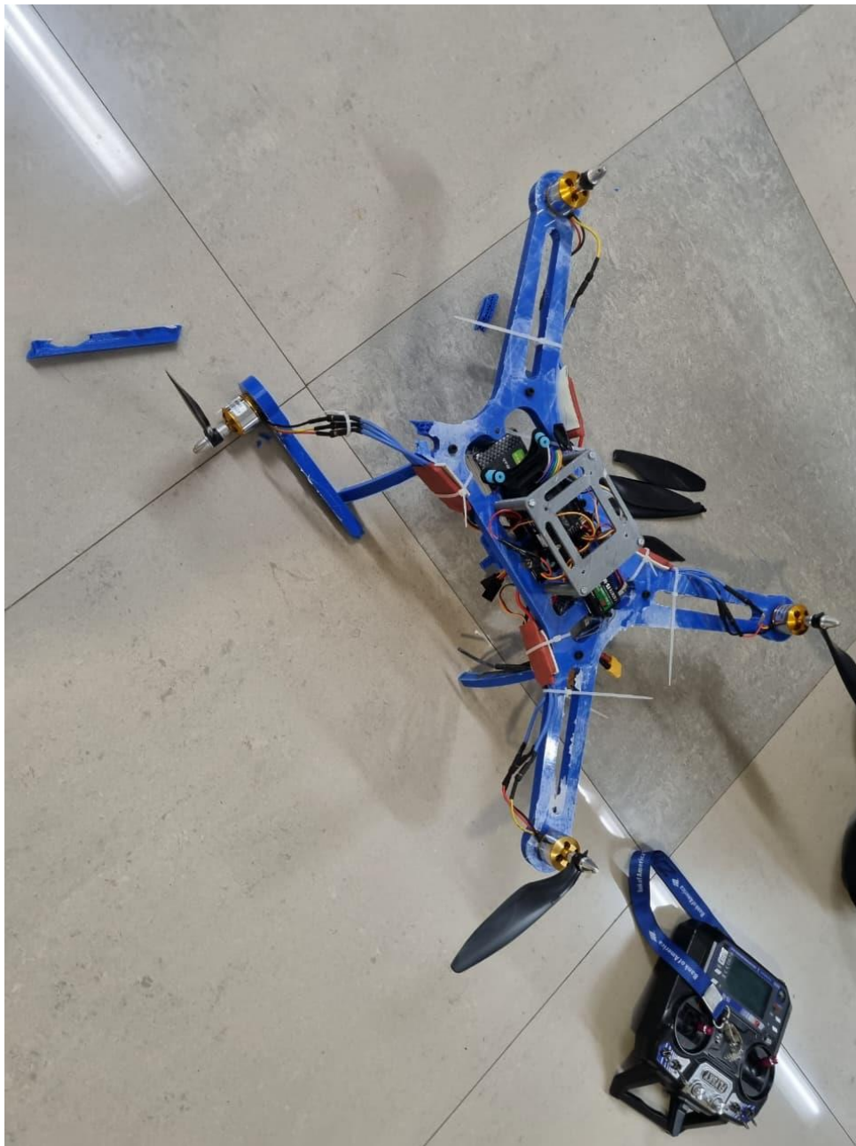
Figure 5. Frame 1 structural failure at arm mounting joint. Clean brittle fracture indicates insufficient internal reinforcement from 10% infill density.
