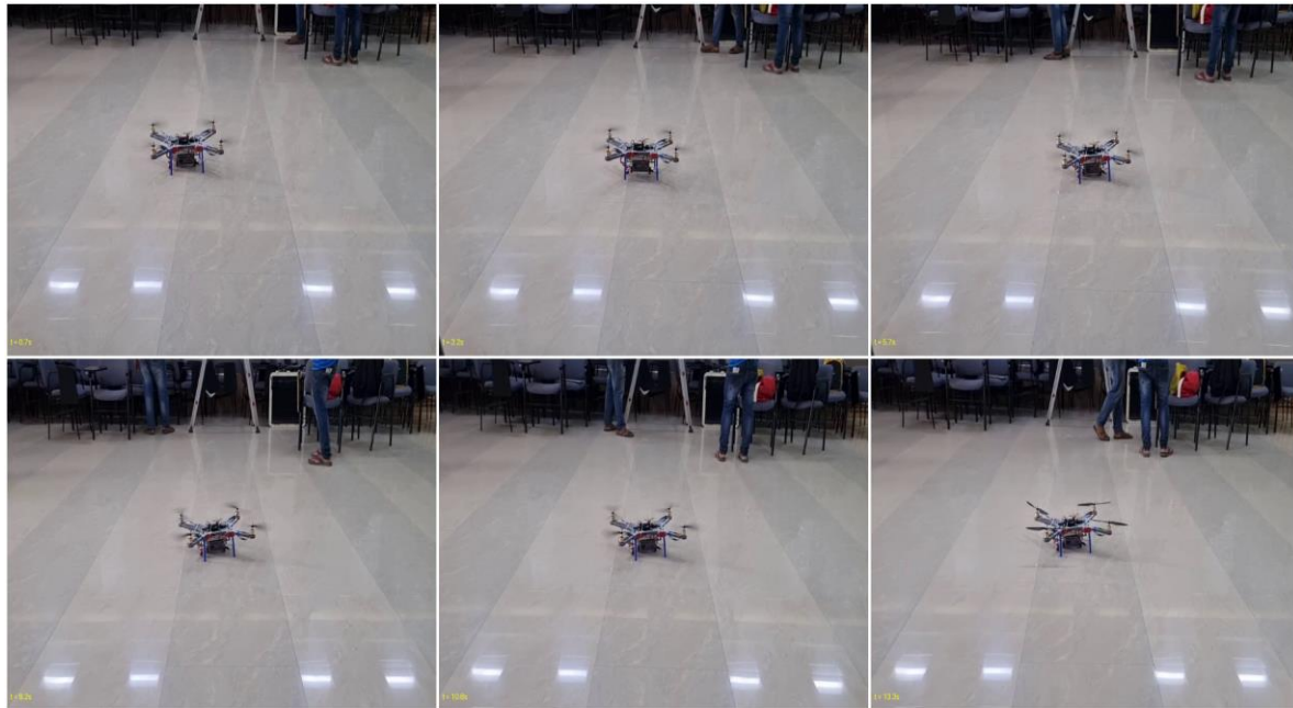
Figure 6. Flight test sequence of Frame 2 (30% infill PET-G). Sequential frames extracted from flight video demonstrate stable hover and controlled maneuvers. No structural degradation observed through 20+ flight cycles.
