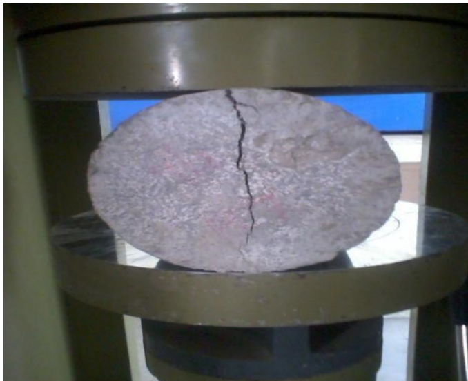
Figure 5. Cracking of ARGFSCC Specimen in Indirect Tension
