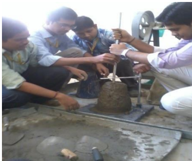
Figure 2. Slump cone test
