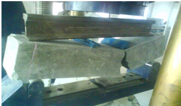
Figure 6. After Failure of Flexure Strength of Prisms on ARGFSCC
