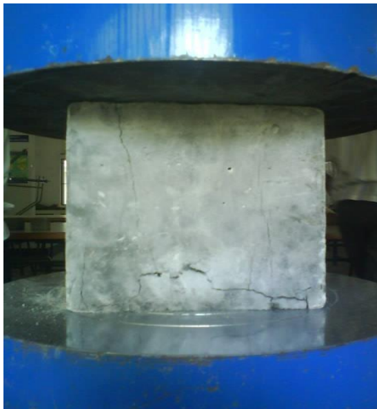
Figure 4. Cracking of ARGFSCC Specimen in Axial Compression
