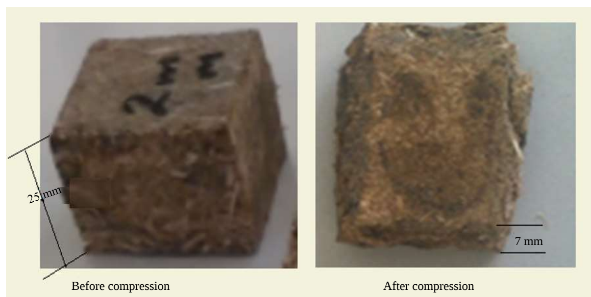
Figure 10. Compression test specimen after and before test.
