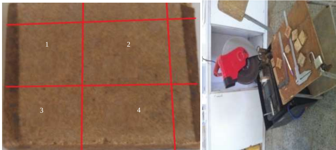
Figure 4. A, B, and C show compression bending and water absorption specimens.
