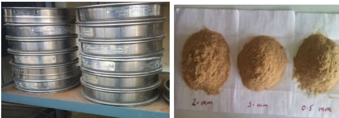
Figure 2. Sieves are used for separation and sample eucalyptus chip particles of sizes 0.5, 1, and 2 mm.
