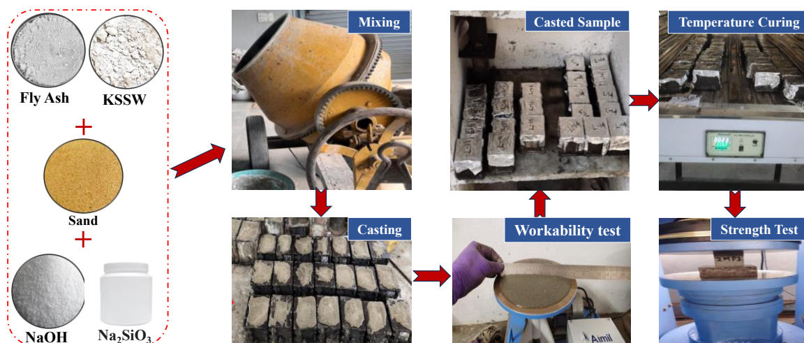
Figure 4. Schematic illustration of material selection, mixing, casting, curing, and testing sequence.
