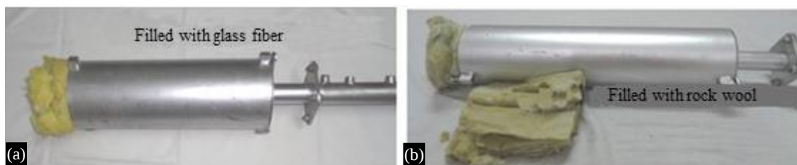
Figure 4. Unfilled muffler compartment consisting (a) Glass wool (b) Rock wool
