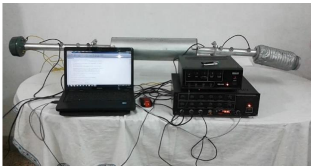
Figure 3. Experimental setup for hybrid absorptive muffler to determine transmission loss under the condition of loading
