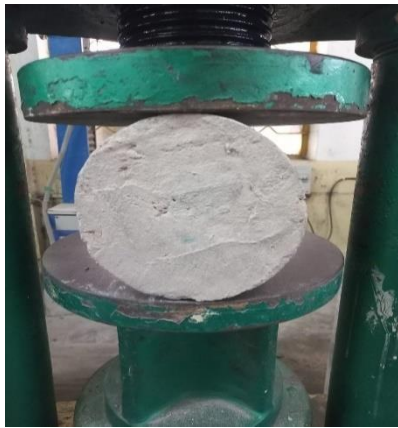
Figure 8. Split tensile test.
