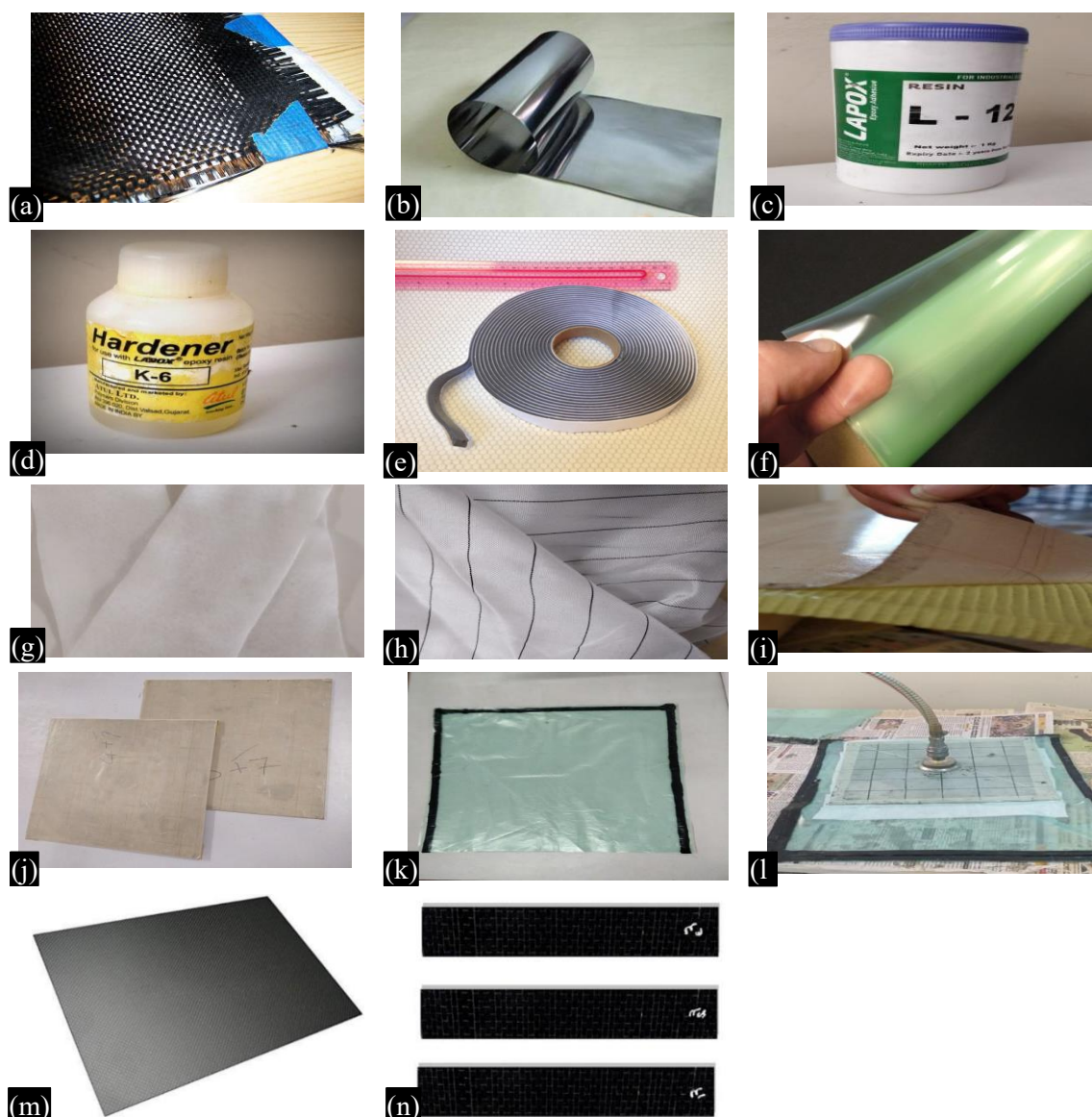
Figure 1. (a–n) From Materials and Components Used in the Fabrication of Titanium-Reinforced Carbon Fiber Composites; (a) Carbon fiber, (b) Titanium foil, (c) L-12 Epoxy Resin, (d) Hardener K-6, (e) Tacky Tape, (f) Vacuum Bag Film, (g) Breather Fabric, (h) Perforated Release Film, (i) Teflon Tape, (j) Moulding Plates, (k) Vacuum bag, (l) Final found out of Vacuum bagging process, (m) Laminates before being cut, (n) Final specimens
