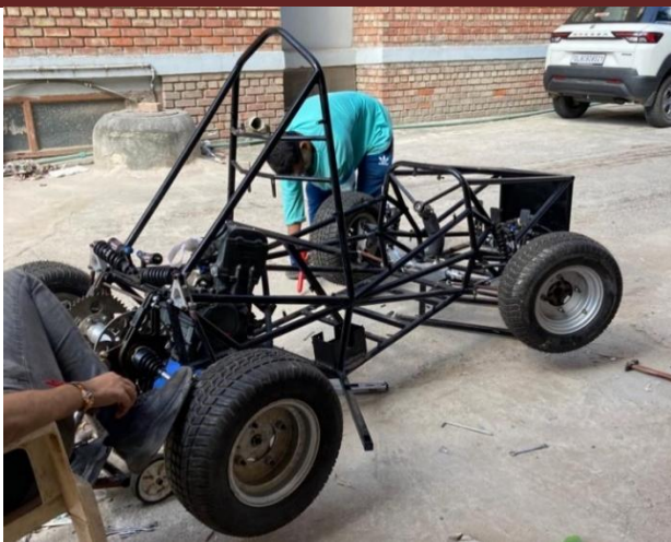
Fig 17 MANUFACTURED CHASSIS AND DRIVETRAIN
