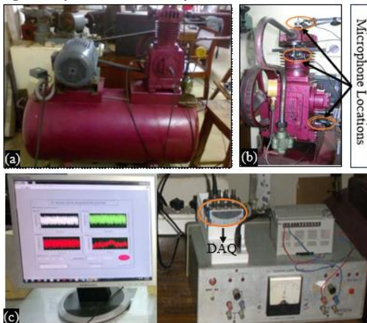
Figure 2. Experimentation: (a) AC system, (b) microphone placements, (c) DAQ [9].
