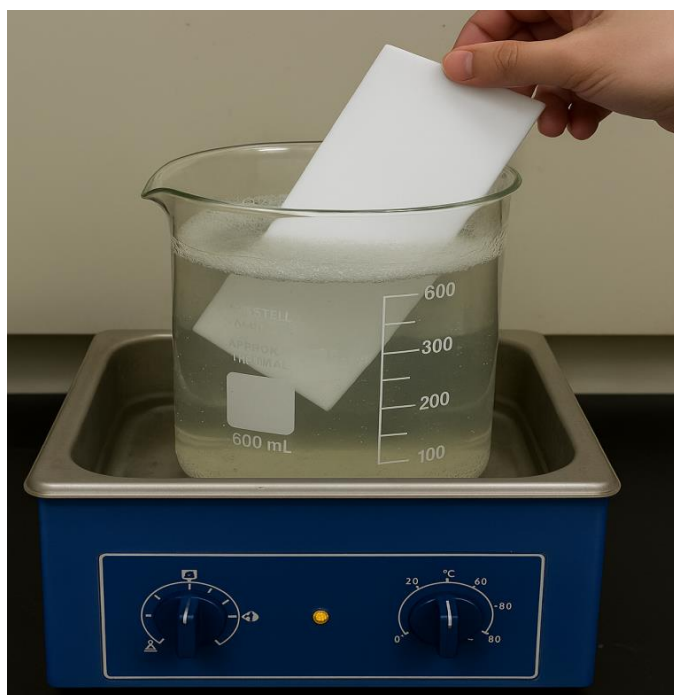
Figure 3. Substrate cleaning via ultrasonic bath.
