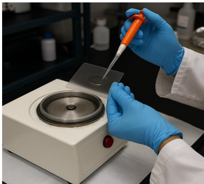
Figure 4. Spin coating of AgNW dispersion on PET substrate.
