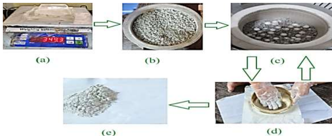
Figure 2. Graphical Abstract of Production Process of Epoxy Micro Particles from Rectangular Blocks. (a) Shows Cross Linked Epoxy Blocks, (b) Shows Epoxy Granules Obtained By Breaking Rectangular Blocks, (c) - Shows Ball Milling of Epoxy Granules, (d) Shows Sieving (At 50 Microns) of Micro Particles and (e) Shows Cross Linked Epoxy Micro Particles. "Author's own Image"
