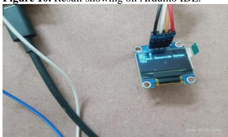
Figure 11. OLED Showing Output of both the Sensors.
