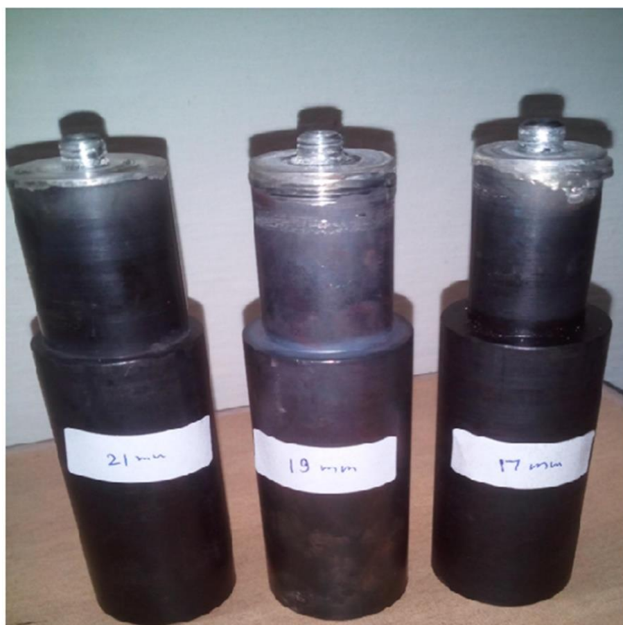
Figure 2. Tool of different shoulder diameters 17 (tool type 1), 19 (tool type 2), and 21 (tool type 3) mm.
