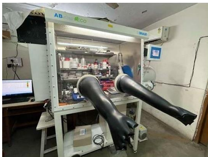
Figure 1. Glove box setup for coin cell preparation.
