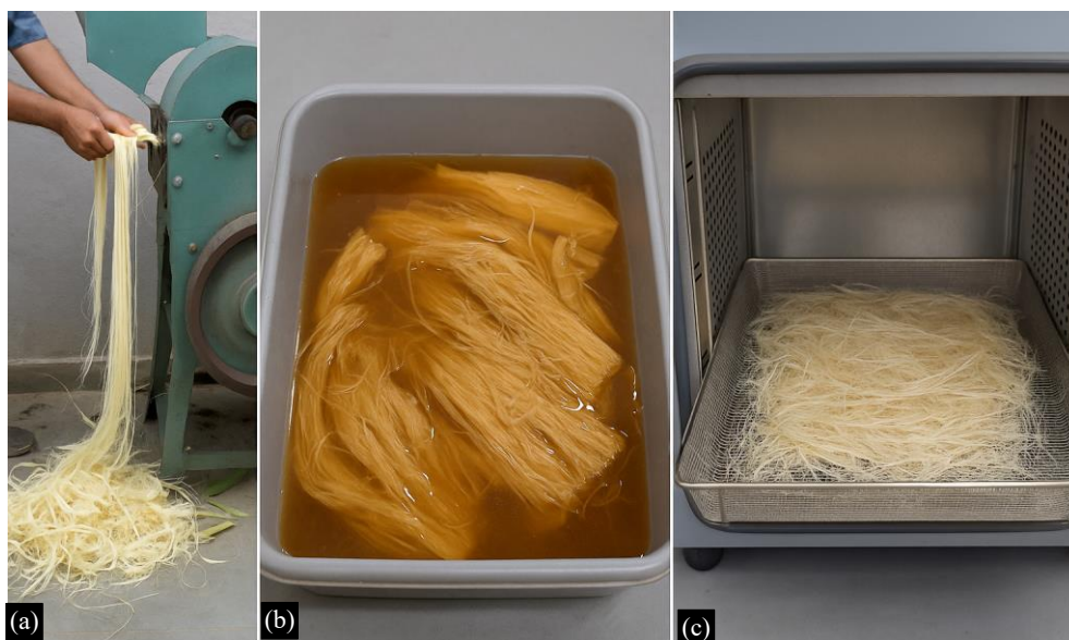
Figure 1. (a): Mechanical decortication of banana pseudostem to extract raw fibers, (b): Alkali soaking of banana fibers in 5% NaOH solution for surface treatment, (c): Oven drying of treated banana stem fibers at 80°C for moisture removal.
