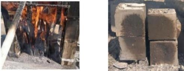
Figure 3. Exposure of fire on concrete cubes
