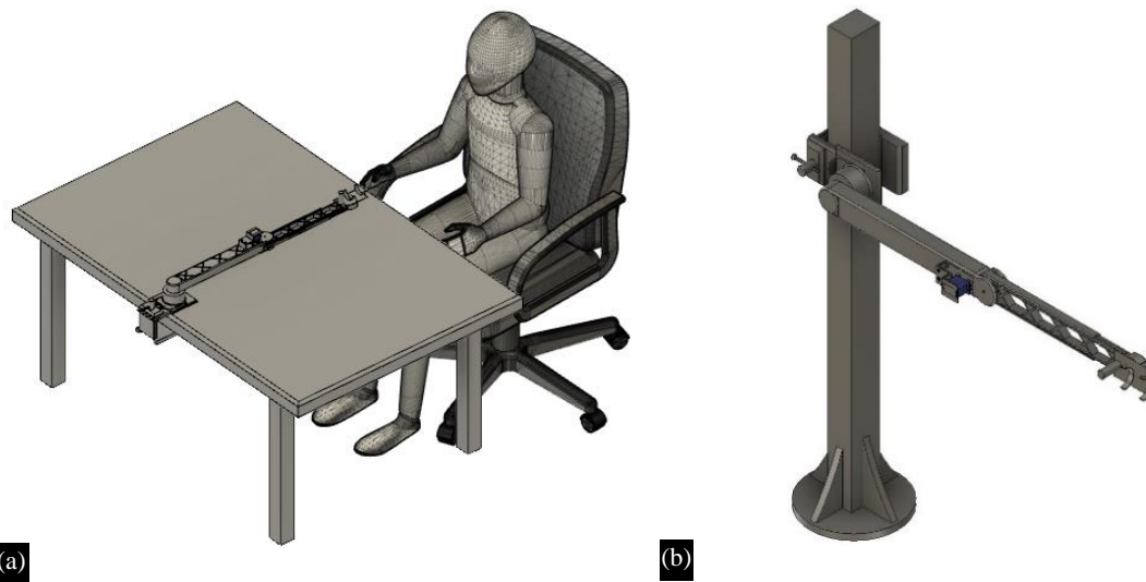
Figure 2. 2R Manipulator for upper limb rehabilitation (a) Tabletop arrangement for Horizontal Plane (b) Vertical pole arrangement for Vertical Plane.
