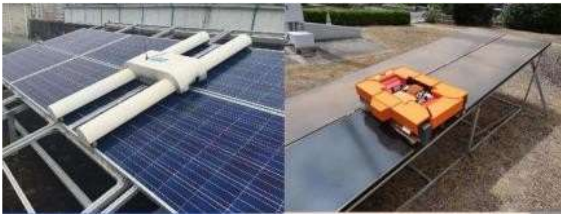
Figure 2. Two main categories of cleaning robot for solar panel.
