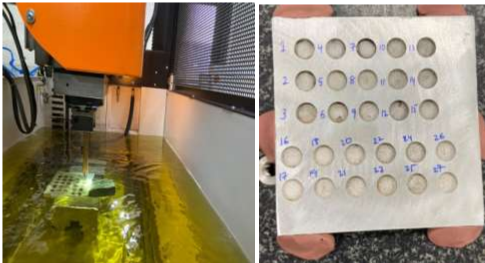
Figure 1. (a) EDM filled with dielectric fluid and immersed specimen (b) Specimen after machining.
