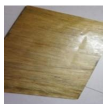
Figure 2. Sample plate after hand lay-up process.
