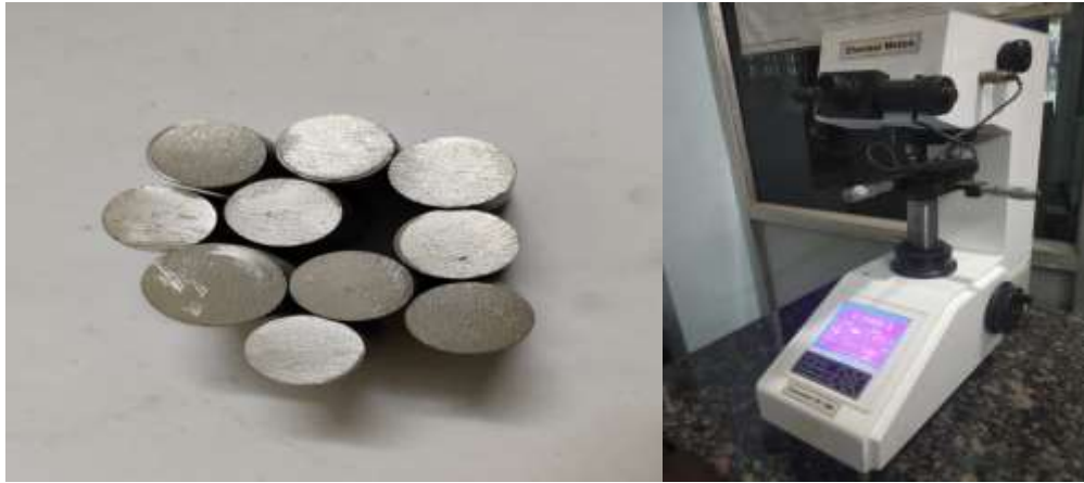
Figure 5. Samples of hardness tests and Micro-Vickers hardness machine
