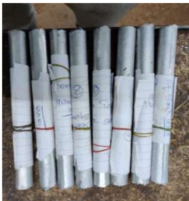
Figure 2. Sand casted specimens after machining
