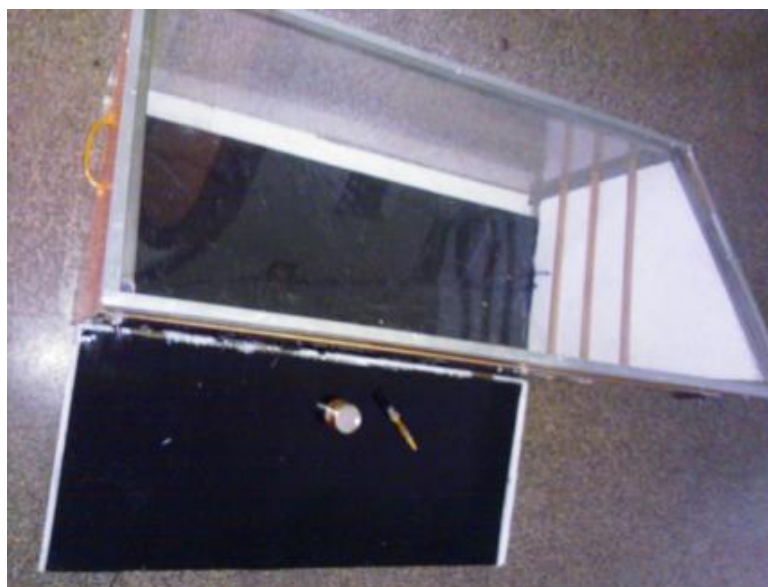
Figure 5. Absorber Plate fixed in the Drying Cabinet
