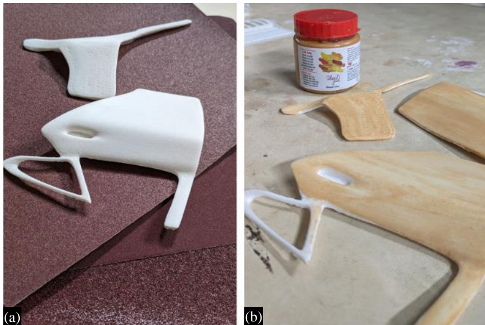
Figure 8. (a) Sanding parts with sandpapers. (b) Applying wood filler and finishing parts.
