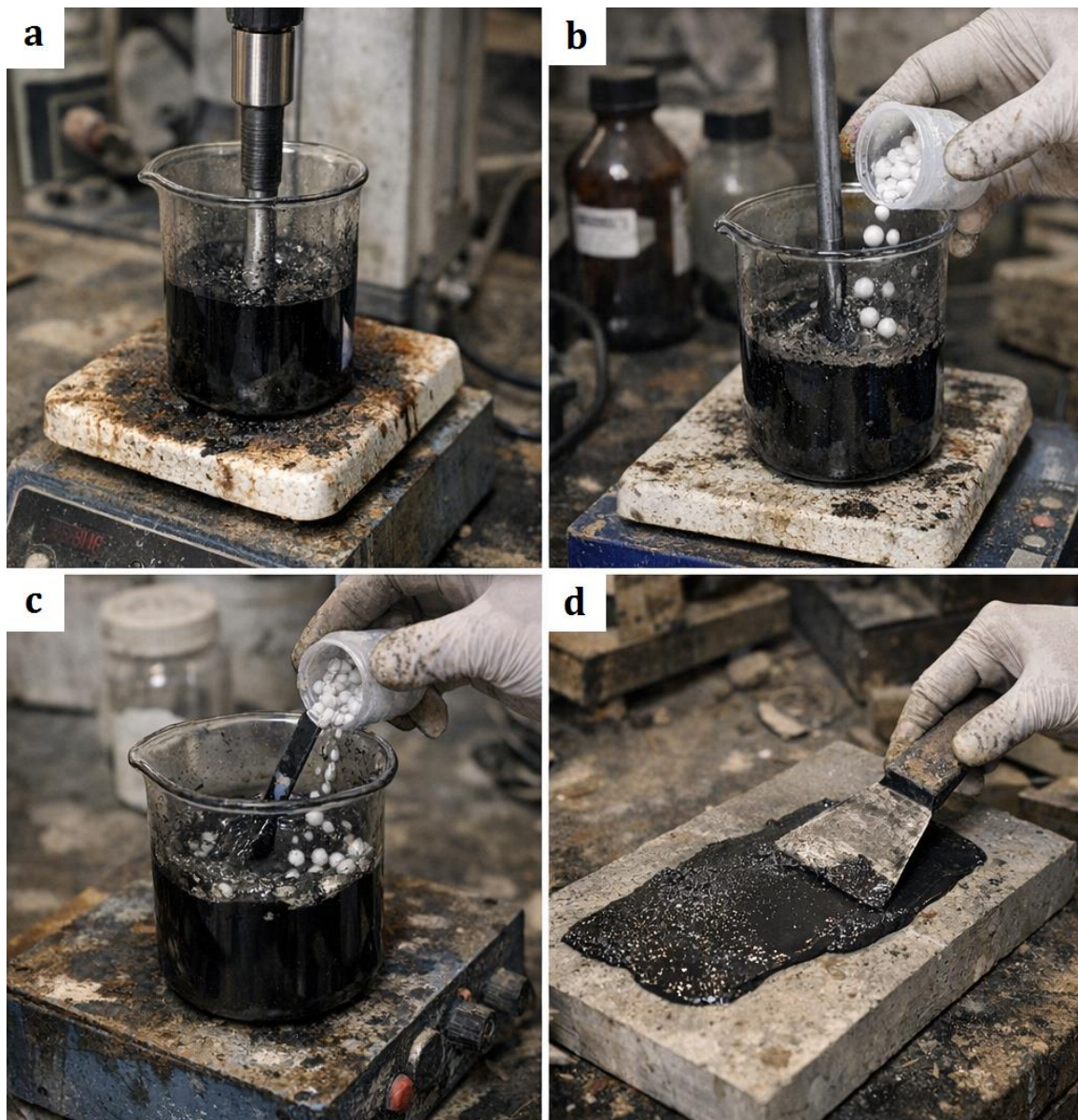
Figure 1. Fabrication of graphene-reinforced polymer composite interface (a) Graphene dispersion in polymer matrix using mechanical stirring. (b) Addition of microencapsulated healing agents into the graphene–polymer composite. (c) Homogeneous mixing of graphene–polymer composite with healing microcapsules. (d) Application of graphene-reinforced polymer composite interface on concrete substrate.
