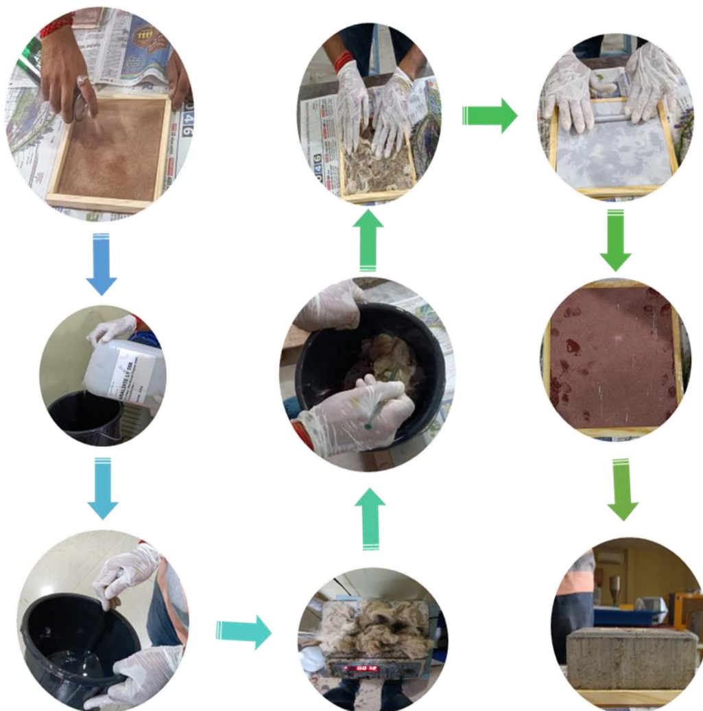
Figure 2. Step-by-step fabrication of hybrid natural fiber-reinforced polymer composite.
