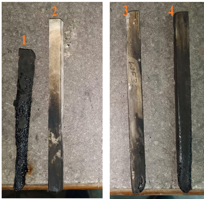
Figure 4. Residual samples after vertical burn test: (1) F5 specimen, (2) W5 specimen, (3) WF32 specimen, (4) WF23 specimen
