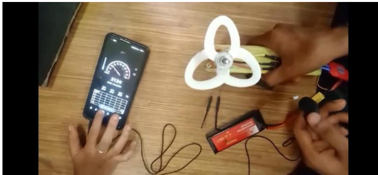
Figure 7. Acoustics noise emission test for the aero propeller using sound meter mobile application.
