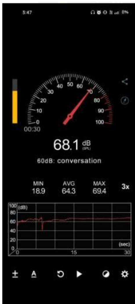
Figure 8. Sample reading using sound meter mobile application for sharrow propeller.
