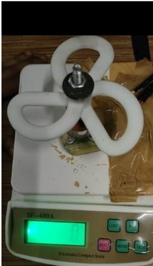
Figure 9. Thrust experiment setup. The sharrow propeller placed over the digital weighting machine.
