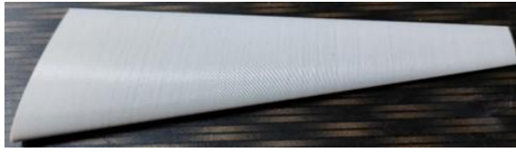
Figure 4 Fabricated model of Un-dimpled 3D aircraft wing
