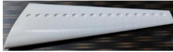
Figure 5 Fabricated model of Inward 16 Circular dimpled 3D aircraft wing
