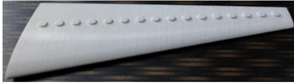
Figure 6 Fabricated model of Outward 16 Circular dimpled 3D aircraft wing
