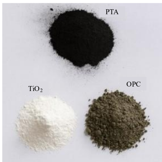
Figure 1. Comparison of palm tree ash (PTA) and titanium dioxide ( \text{TiO}_2 ) with ordinary Portland cement (OPC) used in composite binder systems.
