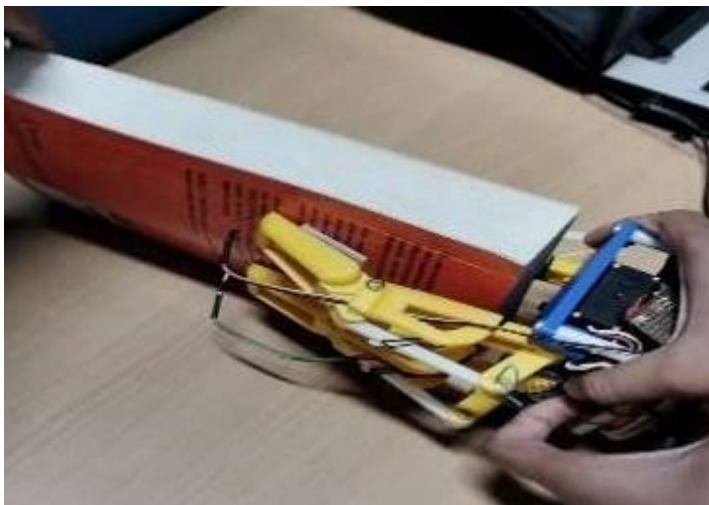
Figure 2. Successfully lifting textbook with gripper picture courtesy. DIAT, Pune.
