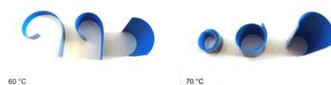
Figure 5. Self-transformation test samples at different temperature.
