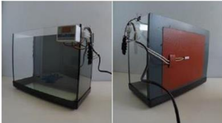
Figure 2. water tank system with a heater and heat controller.
