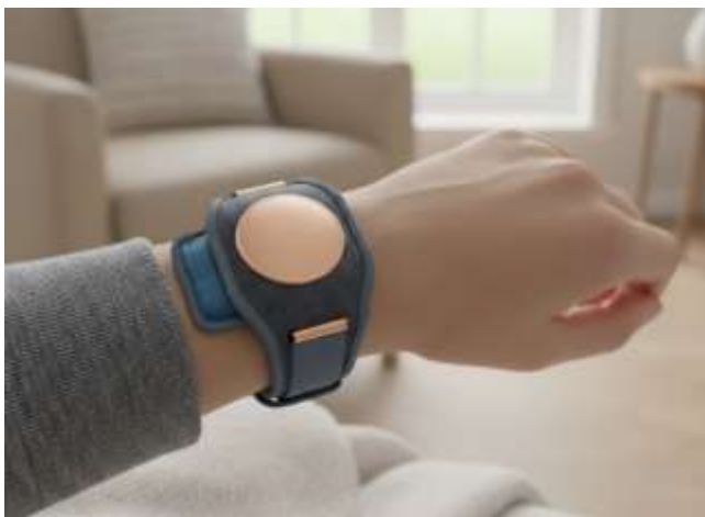
Figure 1. Real life wearable band for migraine detection.
