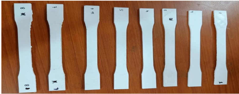
Figure 2. Fabrication of PLA dog bone for UTM for tensile testing.
