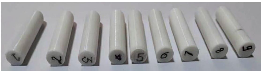
Figure 1. Fabrication of PLA pins for pin-on-disk wear testing.
