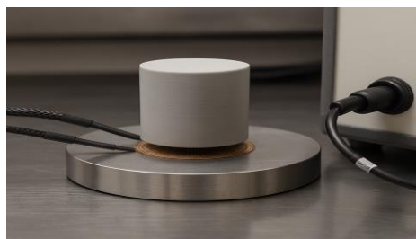
Figure 8. TPS-based thermal conductivity measurement system (ISO 22007–2) using Hot Disk methodology.
