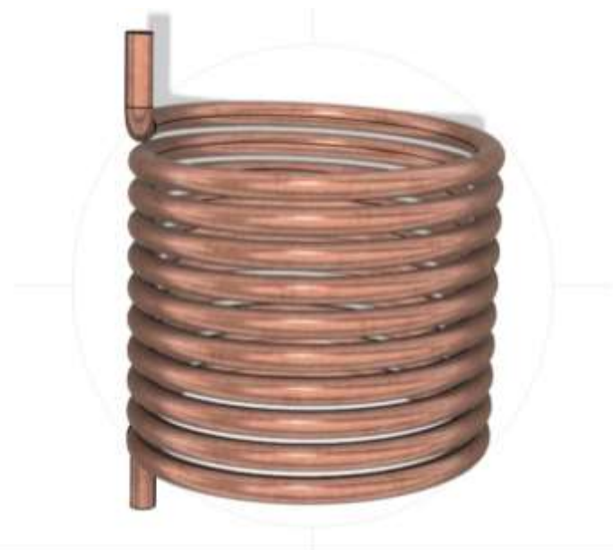
Figure 2. Three-dimensional CAD geometry of the helical coil heat exchanger modelled in ANSYS Design Modeler 2026 R1, showing the continuous helical tube configuration with vertically extended straight inlet and outlet sections. The coil spans approximately 200 mm in the axial direction with a circular cross-sectional tube profile wound in a cylindrical arrangement.
