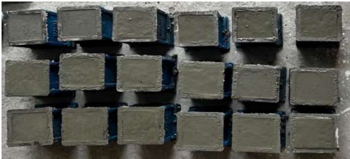
Figure 3. Casting of concrete cubes.
