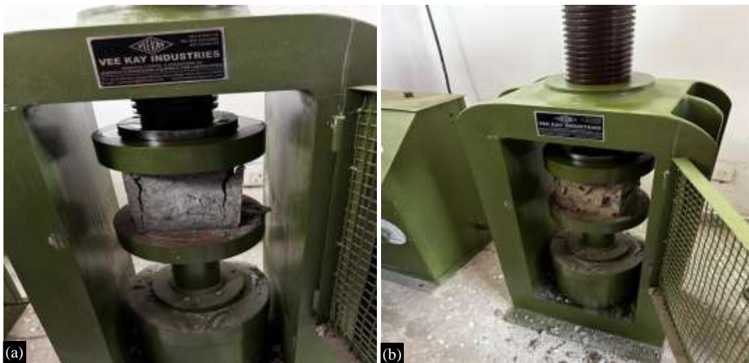
Figure 5. (a) & (b) compressive strength testing of concrete cubes in compression testing machine.
