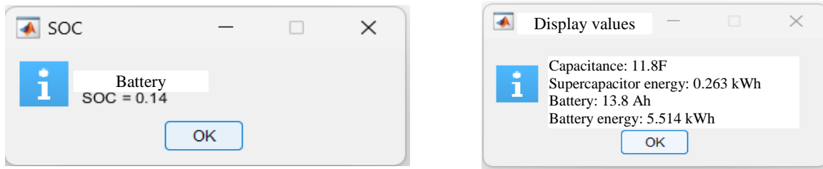
Figure 8. Dashboard information of battery and supercapacitor state of charge at the end of daily route (ECO driving mode)
