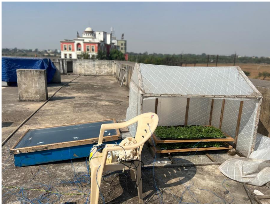
Figure 1. Experimental setup of PV/T-assisted solar dryer.
